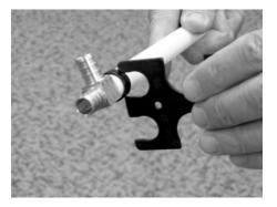
Another type of PEX connection system uses a stainless steel crimp ring to secure the fitting to the pipe. The big advantage to using this method is that one tool works with 3/8", 1/2", 3/4" and 1" pipe. Shown is the *Quickclamp* tool, rings and a few of the many fittings available for use with PEX piping
