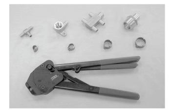
This method is actually easier to use than the ring-type system. Push the stainless crimp ring over the pipe and insert the fitting until it bottoms out. Open the tool completely and place the jaws over the "nub" on the fitting. Squeeze the handles until they close together completely.
